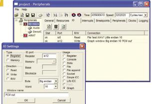
The Project Window instantiates the project and controls the overall debug process. Every processor core in the project is instantiated in the Project Window and has its own list of features and relevant debugging windows. These windows may be managed from the Project Window. The Project Window also contains a logging field as well as a command prompt. Furthermore, clocks, IO, DMA, breakpoint settings as well as interprocessor communication can be setup via this window.
