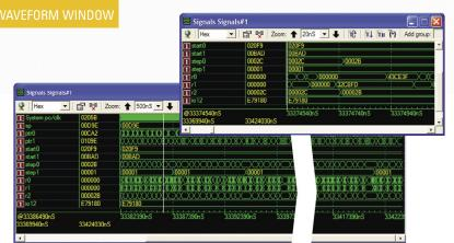
No longer is the Waveform Window restricted to hardware engineers. With Madam Univers, software engineers can now also trace the signal history. In the Waveform Window any value within the ISS of each processor can be traced. This enables the display of the history of selected signals and may give a very good understanding of detailed cycle aspects. It allows to debug and fine-tune the application code.
