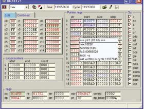
Every processor has its own set of registers, which are displayed in a separate processor Register Window. In addition, the user may build his own customized Register Windows. Besides just viewing the content of registers, it is possible to overwrite these or set various types of breakpoints for each register. The register contents are colorcoded indicating the type of usage of the registers, since last execution.
