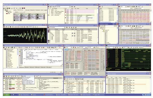
Univers ISSIM's Integrated Development Environment offers the Software Engineer one central cockpit from which he can perform all his code generation and code verification. Univers ISSIM is a multi-processor debugger, which can handle most processors, accompanying tool chains and underlying targets, providing full debug capabilities. Here is a short summary of the main features:
